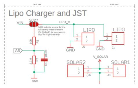
The value of measuring the LiPo voltage is to determine when it is too low to support some power activity.
